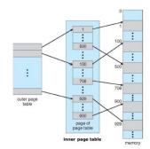
Out goal is to map this structure from kernel space into user space with our own system call. In another word, given a pid of some process A and some virtual address, I need to use my own process "VATranslate" to translate the virtual address into physical address. To complete the mission, I need to use my system call to build my own outer page table and inner page table in my process of user space, while accessing the inner table just gives us the physical address of target process.
