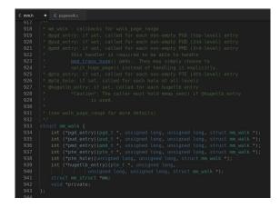
It has several function pointer, which woud be called every time the walk\_page\_range() enter a pgd entry (calling walk->pgd()), a pud entry (calling walk->pud()), … Since our purpose is to remap pte table to user space, and the system has a 2-level page table, we need to accomplish the procedure every time we get into pgd\_entry, and remap the responding pte table touser program.
