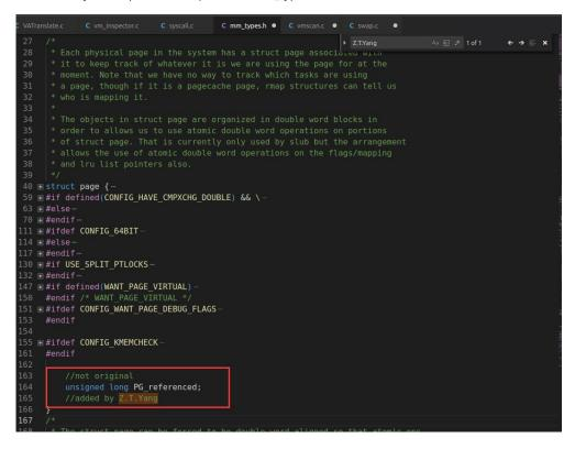
Since originally mark\_page\_referenced() at mm/swap.c was implemented according to 0 or 1 of "PG\_referenced", we change this to shifting right this variable:
