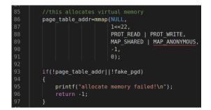
This system call builds a large memory area, but its virtual memory. Use the function remap\_pfn\_rang() in system call "expose\_page\_table" can build a mapping relation of fake inner page table and the "real" inner page table:
